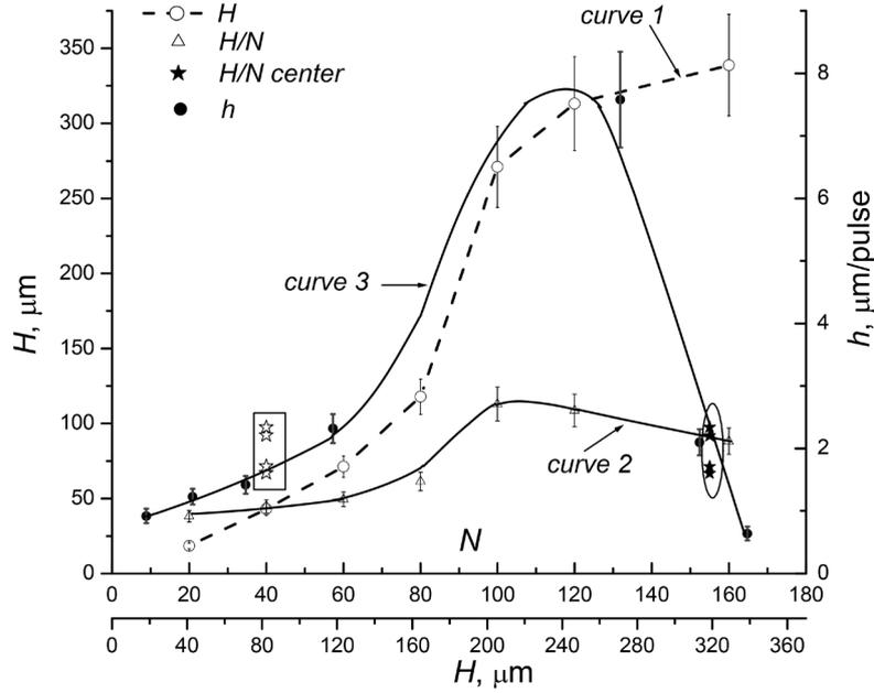
Fig. 2. Dependence of the pit depth  $H$  on a number of  $N$  pulses (curve 1), dependences of the average laser depth ablation rate  $h_{av} = H/N$  (curve 2) and the local laser depth ablation rate  $h_{loc}$  (curve 3) on the pit depth  $H$  at  $F_{213,max} = 0.79 \text{ J/cm}^2$
