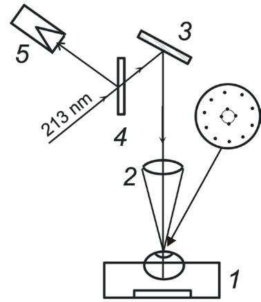
Fig. 1. Optical scheme of the laser ablation research setup: 1 – eye in the holder; 2 – focusing lens; 3 – deflecting mirror; 4 – reflecting quartz plate; 5 – energy meter
