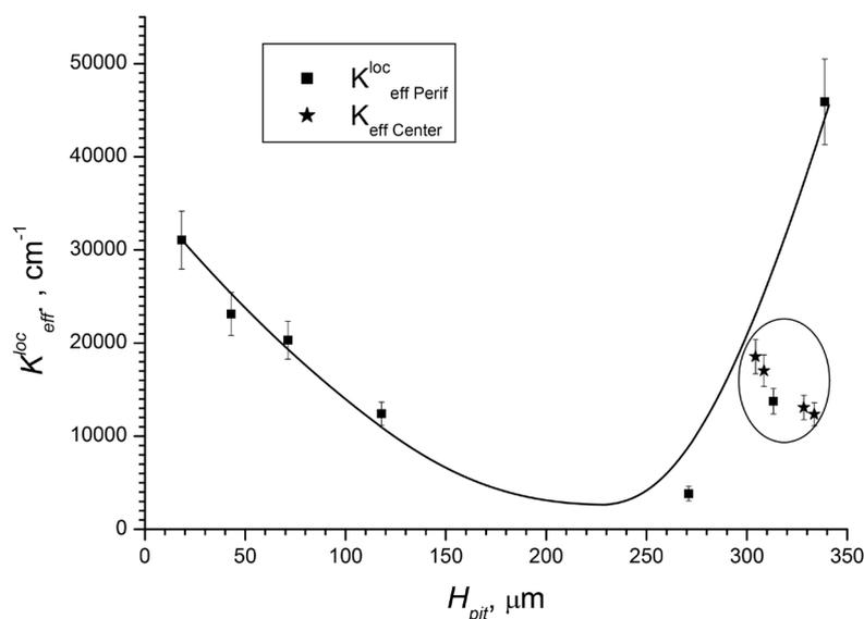
Fig. 3. Effective absorption coefficient  $K_{eff}^{loc}(H)$  as a function of pit depth  $H$  on the periphery and for the pits on the inner radius of the circle (in the ellipse)
