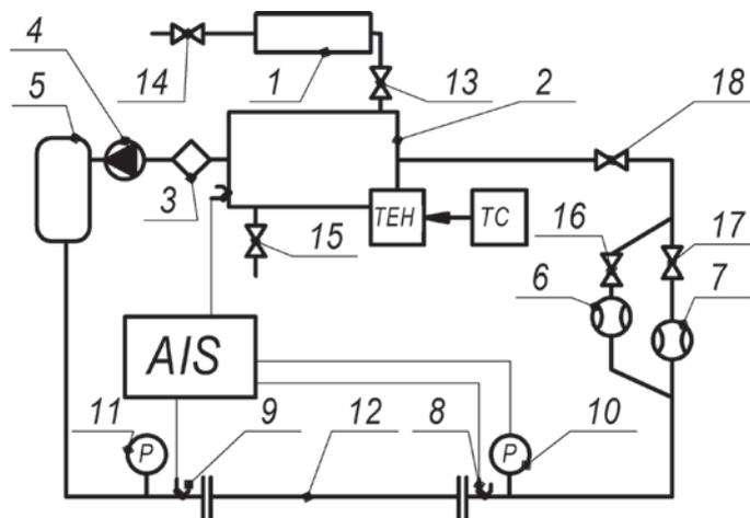
Fig. 2. Test bench for investigation of hydraulic resistance of tubes with internal helical finning: 1 – distiller; 2 – tank-heater; 3 – filter; 4 – high pressure pump; 5 – receiver; 6, 7 – flowmeters; 8, 9 – thermocouples; 10, 11 – pressure sensors; 12 – working section; AIS – automated information system; TEH – tubular electric heater; TC – temperature controller; 13–17 – valves
