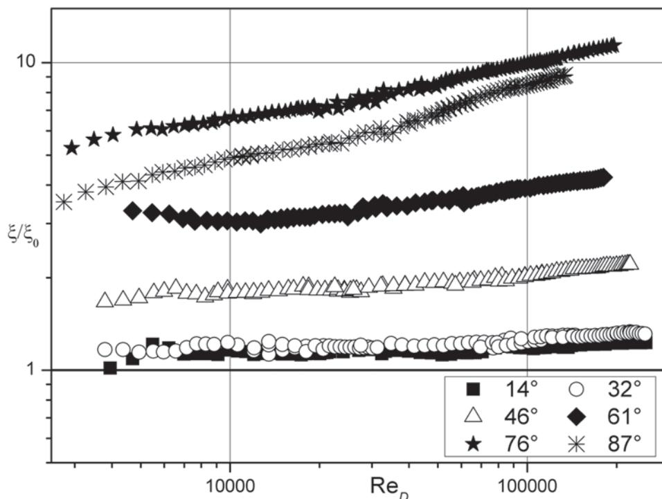
Fig. 4. Comparison of hydraulic resistance coefficients of tubes at different angles of swirling
