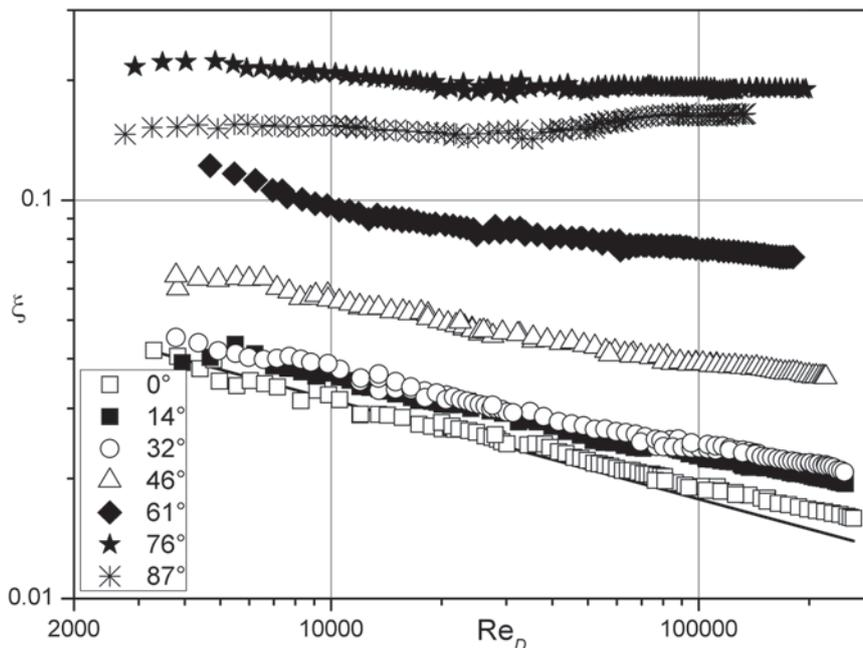
Fig. 3. Experimental data on hydraulic resistance: line – the calculation by the relation  $\xi = 0.3164/Re^{0.25}$  for a tube without internal finning
