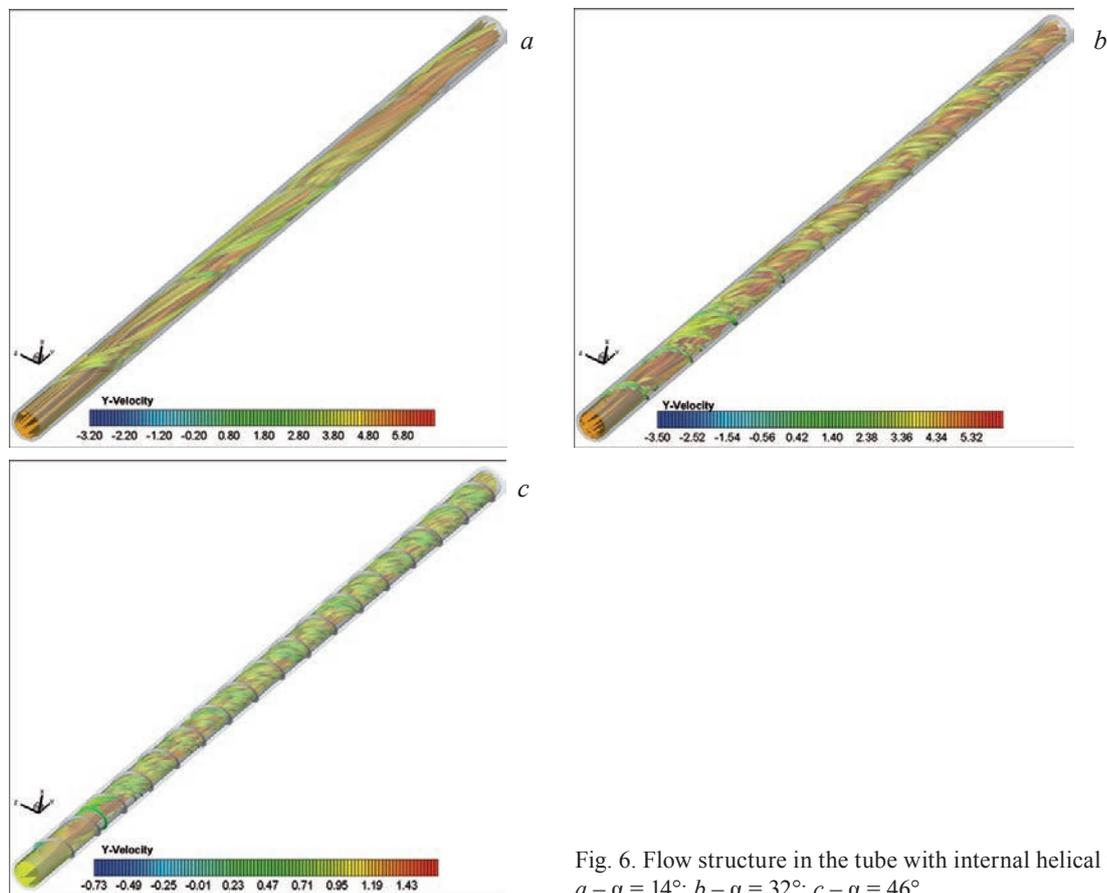
Fig. 6. Flow structure in the tube with internal helical finning:  $a - \alpha = 14^\circ$ ;  $b - \alpha = 32^\circ$ ;  $c - \alpha = 46^\circ$
