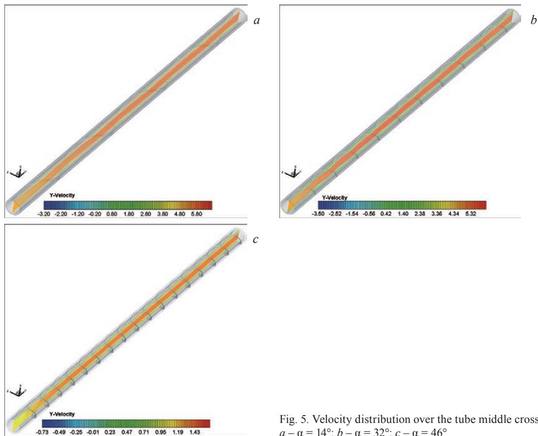
Fig. 5. Velocity distribution over the tube middle cross section:  $a - \alpha = 14^\circ$ ;  $b - \alpha = 32^\circ$ ;  $c - \alpha = 46^\circ$
