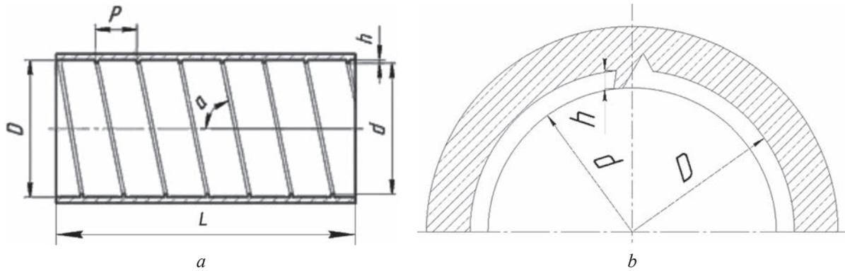
Fig. 1. Longitudinal (a) and transverse (b) sections of tubes with internal helical finning:  $D$  – diameter of a starting smooth tube  $d$  – deformed tube diameter taken from the height of an intensifier (helical protrusion),  $p$  – helical swirling pitch of an intensifier,  $h$  – height of an intensifier (helical protrusion),  $\alpha$  – helical swirling angle,  $\phi = \frac{h^2}{pd}$  – dimensionless parameter responsible for the influence of created swirling on flow characteristics
